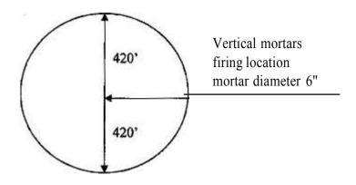
3. The site for the display shall be figured by the largest aerial shell to be fired. If the largest shell is 12"the spectators should be 840ft away, and the secured diameter of the firing site should be 1,680 ft.
